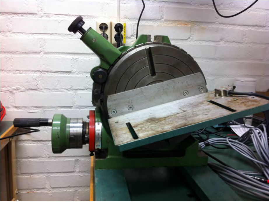
Figure A.9: The rig used for calibration. The inclinometer is fixed at the right side of the rotatable floor.
