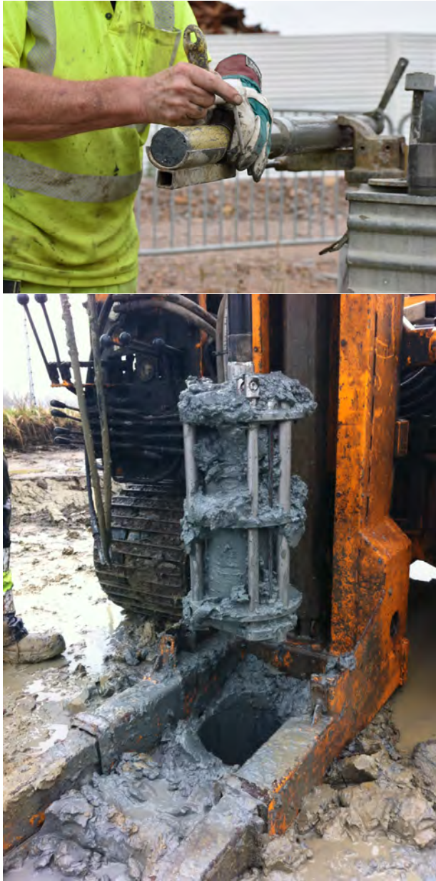
Figure 3.5: Piston Sampling STII, 50 mm diameter, and Mini Block Sampler, with a diameter of 165 mm and height of approximately 300 mm. The soft clay at the test site is easily observed in the photo.
