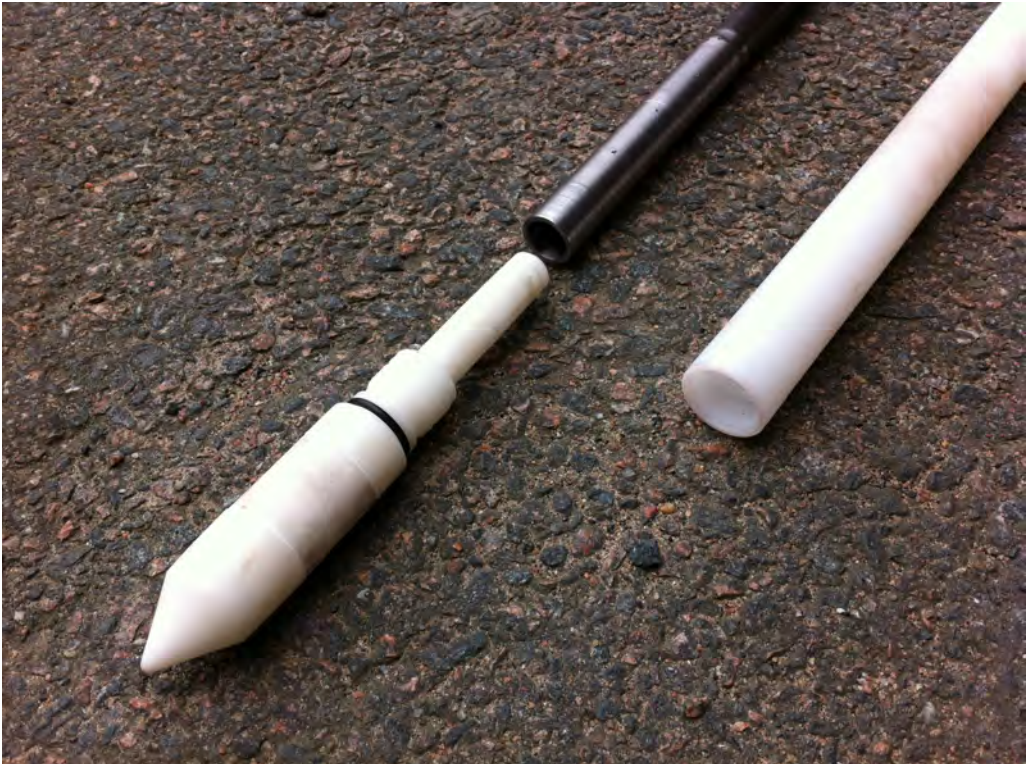
Figure 4.7: Pore pressure and temperature sensor (BAT). Filter tip, plastic pipe and a specially designed installation rod.
